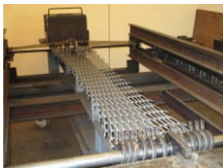
Tensile strength test.
