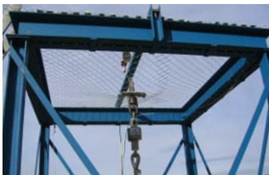
Puncture strength test under "open-air" conditions.
