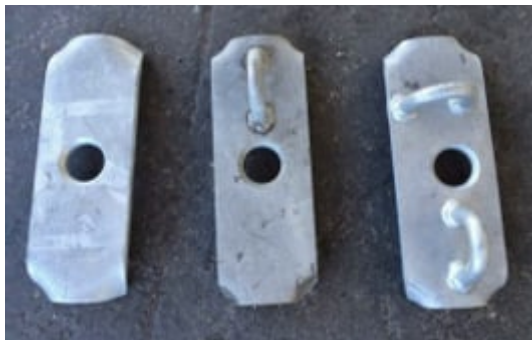
A standard and single and double rope guide spike plates.
