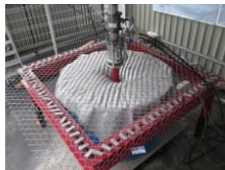
Puncture strength test under "supported" conditions.
